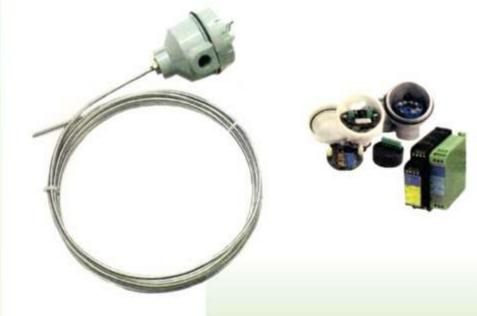
We specialise in manufacturing Mineral Insulated Thermocouples ranging from 1.0 mm OD to 8.0 mm OD, in Simplex as well as Duplex. The above assemblies can be provied with isolated or non-isolated junctions & terminations with flame proof head, Quick-Disconnect type connectors, spring loaded block, etc or flying leads. The Sheathing of the assemblies are available in various materials like SS 316, Inconnel 600, Ss310, etc.
